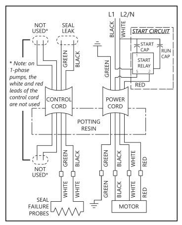
Figure 1. Wiring Diagram 1-Phase
