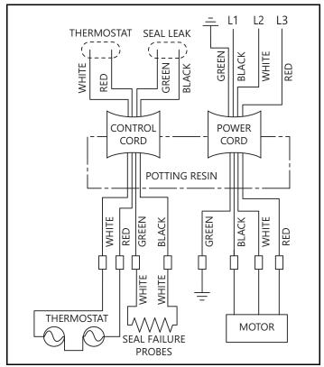
Figure 2. Wiring Diagram 3-Phase
