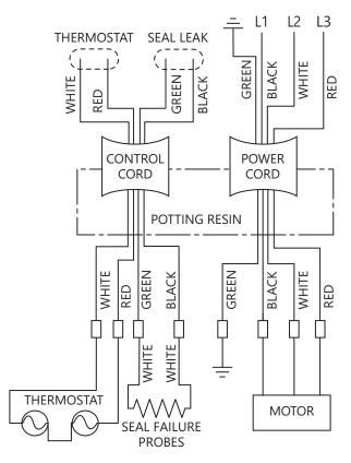
Figure 2. Wiring Diagram 3-Phase
