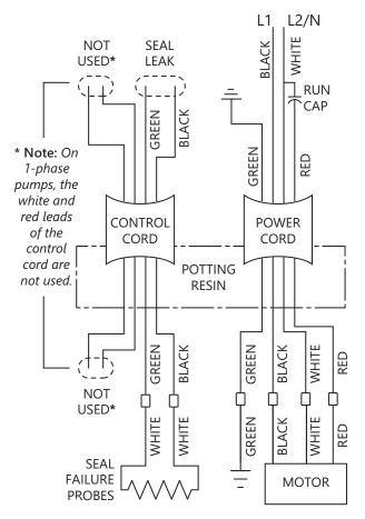
Figure 1. Wiring Diagram 1-Phase
