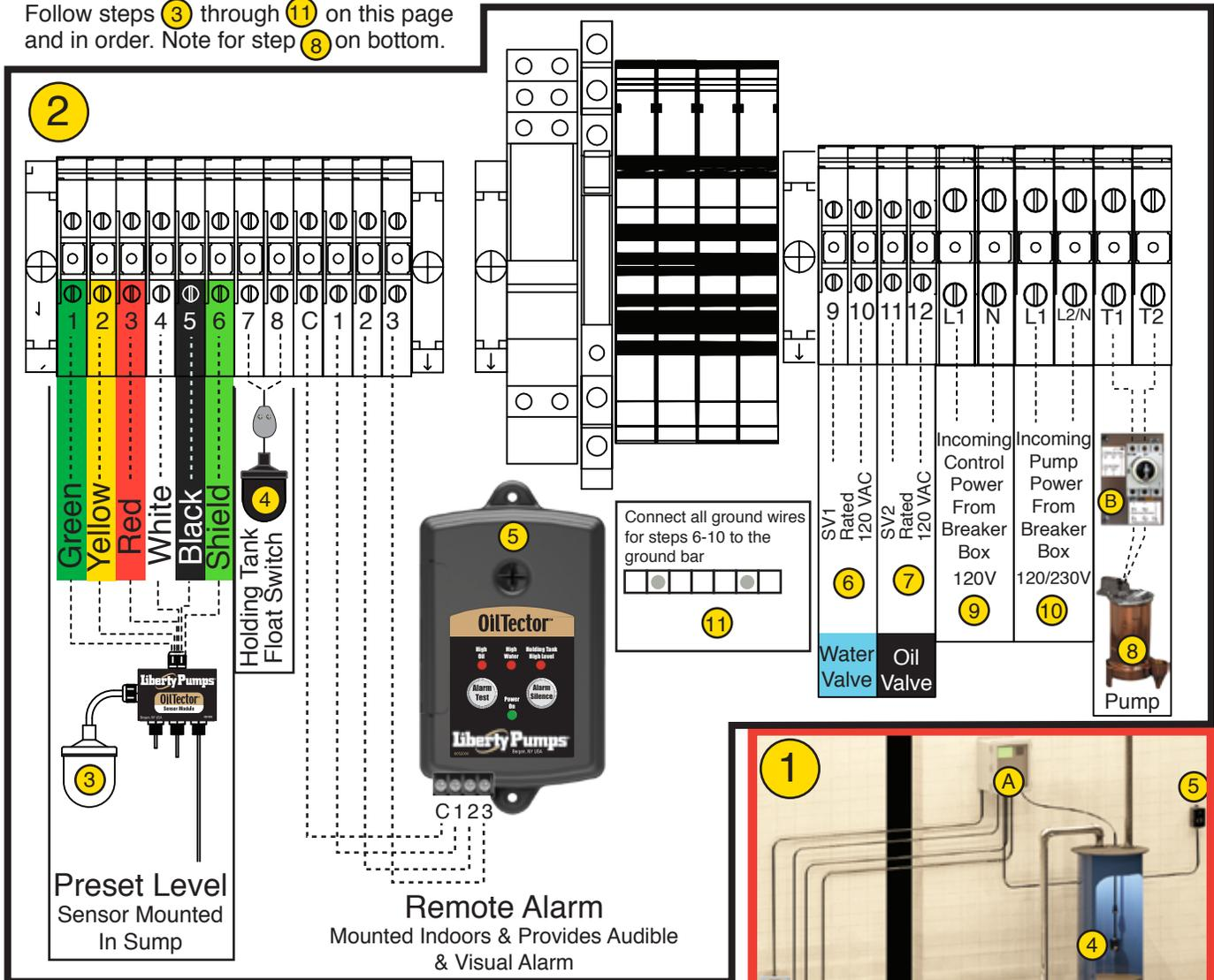
Note: The pump **8** is wired to the bottom of the disconnect switch in the junction box **B** then the top of the disconnect switch in the junction box is wired to the control panel **A** Terminals T1 & T2.
