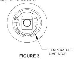
The main handle of the Temp-Gard III value is for temperature control only. To turn value on, the handle is turned counterclockwise through the cold position, to the warm and then to the hot position. The range of motion on the handle is 140°.
