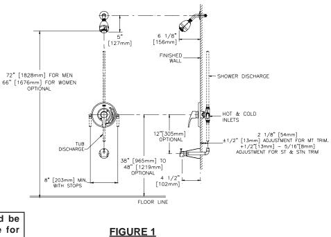
FOR OPTIMUM VALVE PERFORMANCE, BALANCE SUPPLY PRESSURES TO LESS THAN 5 PSI PRESSURE DIFFERENTIAL BETWEEN HOT AND COLD WATER SUPPLIES.
