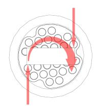
EDGE ENGAGEMENT: 80 FT-LBS TOOL ENGAGES VALVE KNOB EDGE MINIMIZING PINS ENGAGED.
