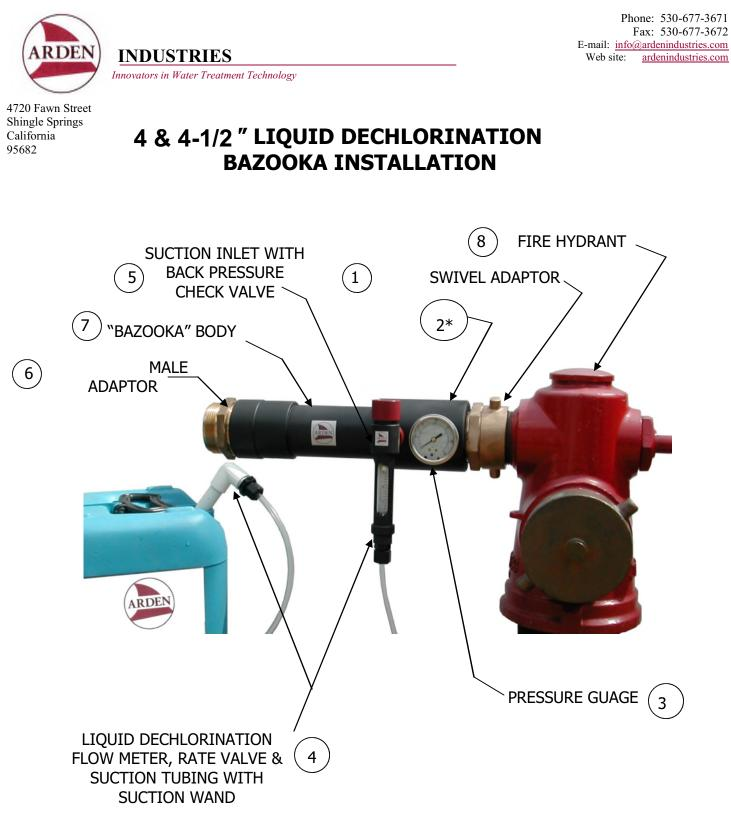
NOTE: 1. This is a typical installation for flushing through Fire Hydrants. Units can also be attached to  $2-2 \ 1/2''$  Risers from Water Mains for flushing super chlorinated water.
