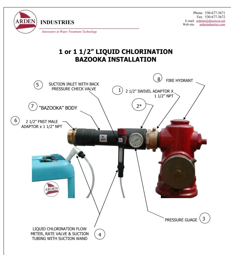
NOTE: 1. This is a typical installation for flushing through Fire Hydrants. Units can also be attached to 2-2 1/2" Risers flushing Super Chlorinating Water Mains..
