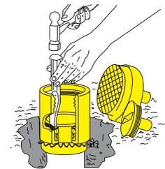
Fig. 6 Inside Caulk Outlet C
