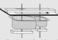
Above shows how threaded rod and timber bearers may be used to clamp the sink in place while fastening to the counter / benchtop using methods B and C.
