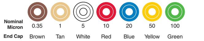
Graph colors (left) correspond with color codes (above) used to identify nominal micron rating of cartridge.
