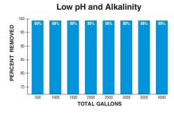
Test data generated by certified national laboratory using the protocol described in NSF Standard 53 using a flow rate of 0.75 gpm and an average feed of 150 ppb lead. Water's pH was 6.5 and alkalinity 10-30 ppm as CaCO<sub>3</sub>.
