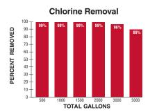
Test data generated by independent laboratory at 1 gpm using test procedures described in NSF Standard 42. Average chlorine feed at 2 ppm.
