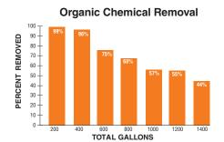
Test data generated by independent laboratory at J gpm using test procedures described in NSF Standard 53. TCE used as test contaminate at average feed of 300 ppb.
