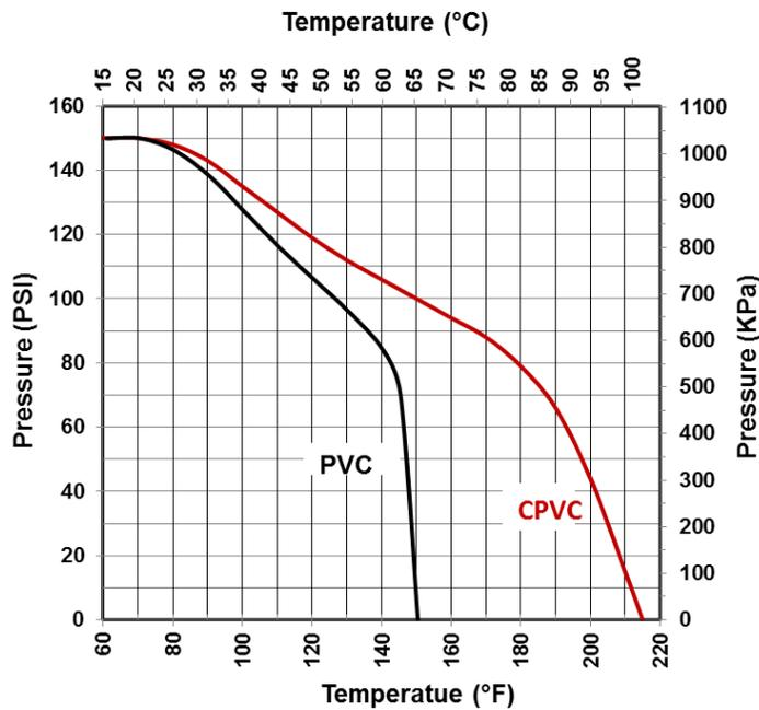
**Graph 1: Operating Pressures of PVC and CPVC Materials at Elevated Temperatures.**
