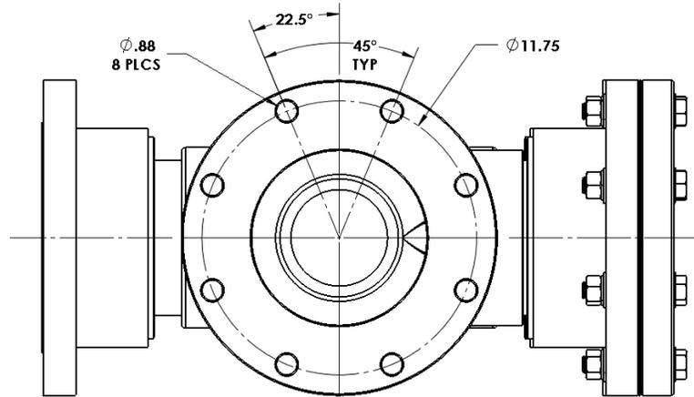
Figure 1: SB Series 6" & 8" Base, Bottom View
