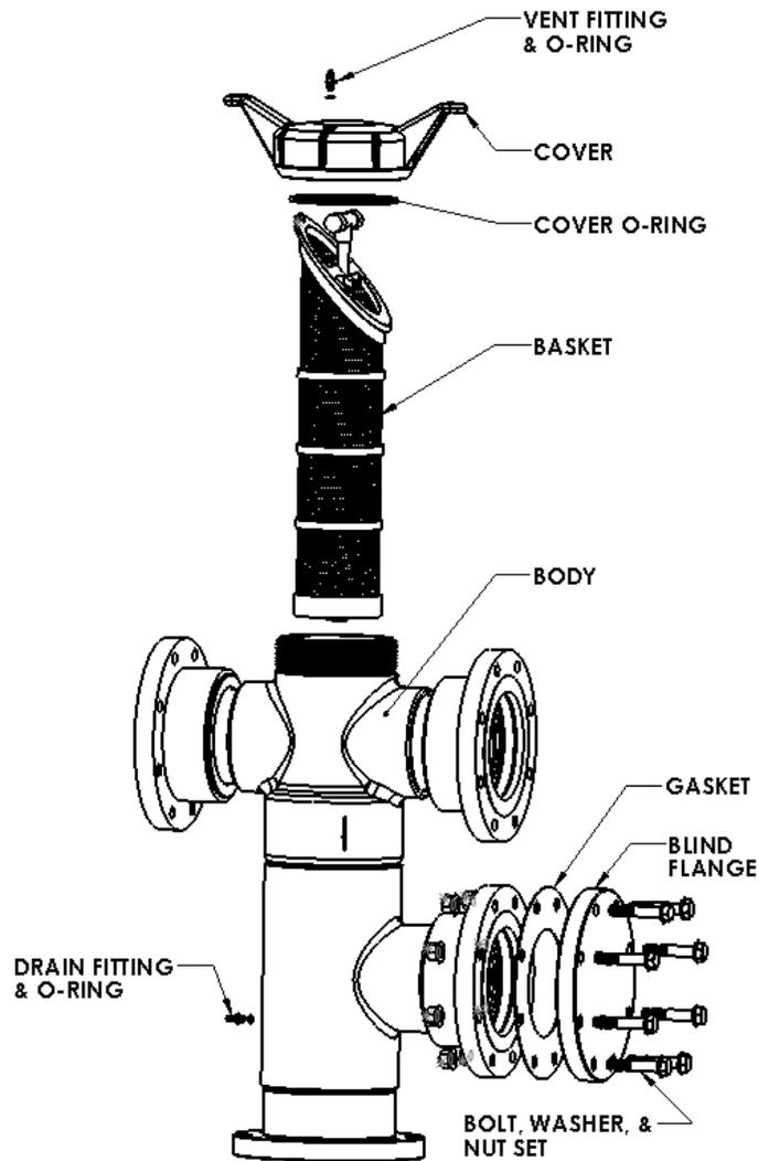
Fig. 5: Exploded View of 6" & 8" PVC and CPVC SB Series Strainer Basket Assembly
