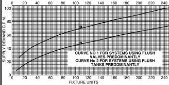
The Graph Chart is based on the U.S. Bureau of Standards Sizing Table and may be used to determine the fixture unit rating based on GPM supplied to the fixture in auestion. HYDROTROL SIZING CHART
