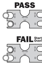
**STEP 4** BE SURE TO CHECK EVERY CRIMP JOINT! Every crimp joint should be checked with the GO/NO GO Gauge. If the designated GO slot fits over and will rotate around the crimped ring, you have made a proper crimp. If the crimped ring will fit in the NO GO Gauge or will not fit in the GO Gauge, you must cut the crimp joint off and make a new connection.
