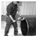
beveled on the outside extreme end after cutting. A portable grinder should be used to make a bevel 3/8" to 5/8" long at an angle of 30-40° with the axis of the
