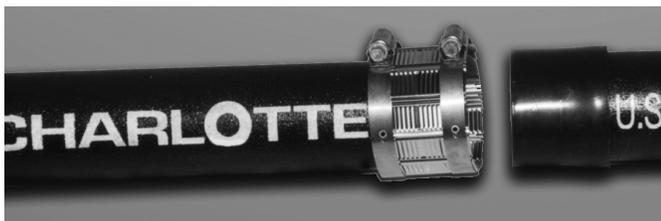
2. Place the neoprene sleeve on the end of the pipe or fitting, firmly seating the pipe or fitting end against the integrally-molded shoulder inside the sleeve. Also place the stainless-steel shield on the other component you're joining. Note: If you are working with a fitting, make sure the neoprene sealing sleeve makes contact with its positioning lug.
