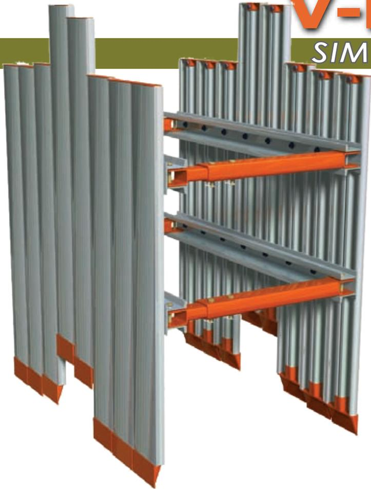
V-Panel is a box that is easy to lift and move around on the job site. Use the versatility of the movable Shore panels to work around existing utilities or T-off from your main trench in safety. Protect your workers at each end of the box with the variable width durable panels. As a shoring system, the vertical panels stop ground movement to protect adjacent structures.
