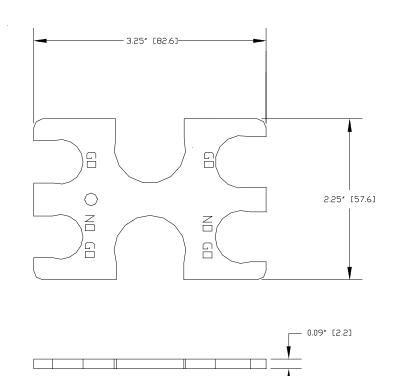
**Engineering Specification:** Zurn Go/No Go crimp guages. QGA234P can be used to check 3/8", 1/2", and 3/4" crimps.
