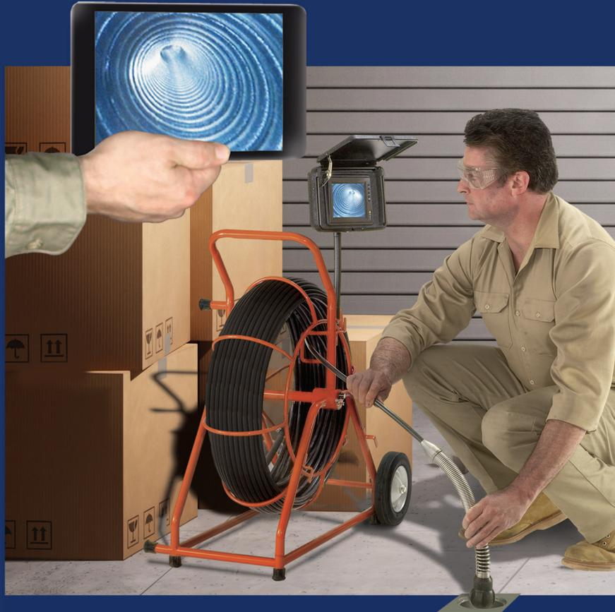
Patented Gel-Rod push rod withstands tough abuse in the line. The Gel in the rod keeps moisture away from the wires inside if it's ever cut or abraded. Dual layer/dual color construction let's you see rod wear so it can be repaired before it becomes a problem. Kevlar braid, fiberglass core and durable sheath provide maximum pushing and pulling power.
