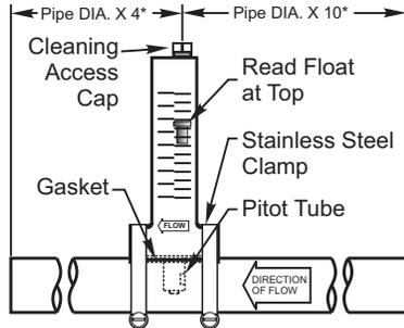
\* Minimum acceptable dimensions. Must be straight horizontal piping.
