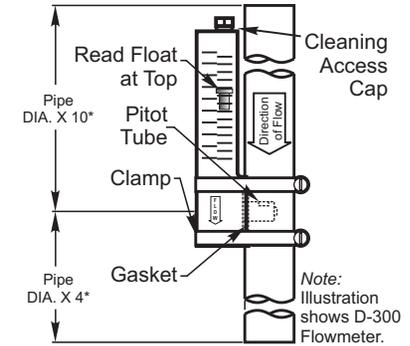
\* Minimum acceptable dimensions. Must be straight vertical piping.
