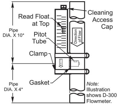
\* Minimum acceptable dimensions. Must be straight vertical piping.
