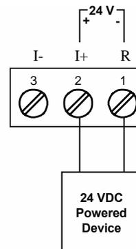
Figure 23. Analog Output Supply Powering Other Devices
