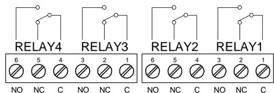
Figure 18: Relay Connections
