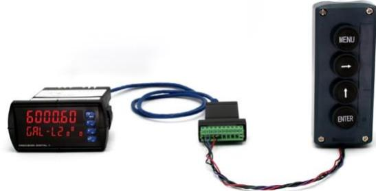
Figure 27. Meter to Control Station Connection
