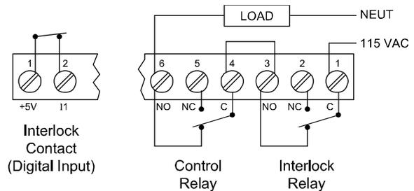
Figure 28: Interlock Connections
