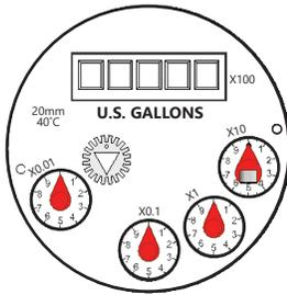
The **3/4" meter** has a fourth dial, as shown above. The x0.01 dial is used for 20 P/G and 10 P/G rates. Note: The 3/4" meter has a 5 digit totalizer.
