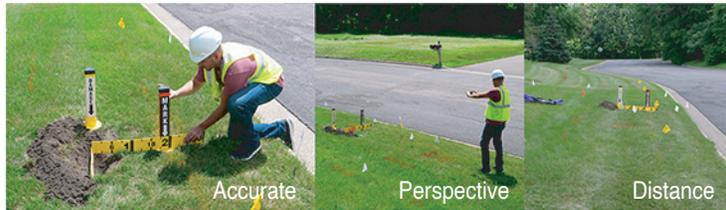
The Rhino HIT Kit™ is used to enhance root cause investigations and to accurately record damage to buried facilities such as fiber optic cable, pipelines, electrical lines, and more. It enables consistent photographic damage reporting by using a standard tool to record every accident which can reduce unnecessary and costly legal actions when damage occurs. \*For larger damage investigation areas check out our HIT Kit+2™.
