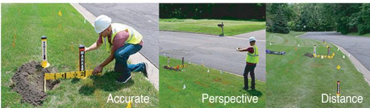
The Rhino HIT Kit +2™ is used to enhance root cause investigations and to accurately record damage to buried facilities such as fiber optic cable, pipelines, electrical lines, and more. Use of the HIT Kit +2™ allows for consistent photographing of a large area for damage reporting by using a standard tool to record every accident which can reduce unnecessary and costly legal actions when damage occurs. It also assists in identifying locate marks for a clearer depiction of the scene.
