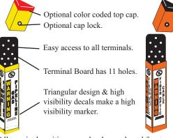
All terminal positions are clearly numbered front and back (1-11) to assist with internal documentation, installation and testing. Each terminal is spaced 1" on center to allow easy use of shunts for cathodic protection or continuity bridges for tracer wire applications. The design of the molded UV stable terminal board allows easy installation of wires and will not become brittle or break even in extreme cold temperatures. The removable cap protects the terminals from the elements.
