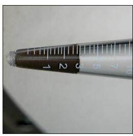
Includes six polycarbonate 19mm diameter conical bottom tubes. Clearly marked for solids concentration in percent volume as low as 0.20%.
