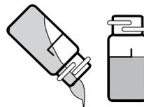
10. Use the 0.5 mL pipet [0353] to add 0.5 mL of \*Sodium Arsenite Solution [4128]. Cap and mix.
