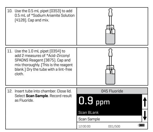
NOTE: Zeroing the meter with the sample water will result in an error. Meter must be zeroed with a reagent blank.
