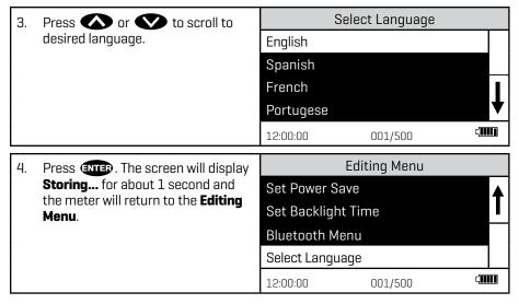
NOTE: If meter unintentionally switches to another language, use the procedure above to reset the meter to the desired language. For example, to reset the meter to English:
