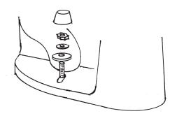
Install the toilet tank. (The tank has been factory assembled and has the gasket seal between the bowl and the bottom of the tank and is ready to set in place.) Place the tank on the toilet bowl. Slide the tank toward the front or back of the bowl until the desired gap is obtained between the tank and the wall. (Note: the gap is normally 1/2- to 1-inch.) Secure the tank in place with the two (2) metal washers and (2) wing nuts provided. **DO NOT OVERTIGHTEN.**
