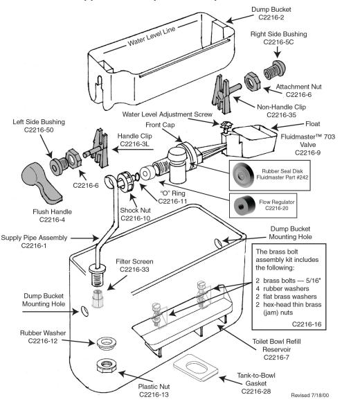
\*Left-hand assembly of flush handle components shown in shaded areas; reverse these parts for right-hand flush handle assembly.
