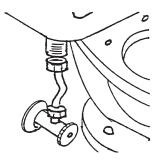
Open the shut-off valve slowly and check for leaks. Fill the Flapperless<sup>TM</sup> dump bucket to the water line. Adjust the level, if necessary, by turning the black screw on top of the float. Turn the screw to the right to lower the water level or to the left to raise the level.
