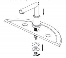
Slide Hot and Cold end valves thru sink mounting holes. Make sure long tubes are installed facing away from spout. <u>Note: Hot side end valve is labeled.</u> Secure end valves with washers and nuts. Hand tighten nuts onto shank. Lock nuts into position by tightening screws.
