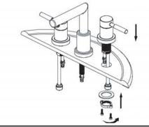
Align tabs (1) and (2) on quick connects (3). Push quick connect housing firmly upward and snap onto receiving tube tab. Pull down moderately to ensure connection has been made. If it is necessary to remove quick connect, squeeze tabs on hose between index finger and thumb, then pull down to disconnect.
