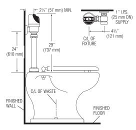
The Model 8115 valve is designed for installations where the water supply is roughed-in 24" (610 mm) above the top of the water closet. For new installations, Sloan strongly recommends the use of our Model 8111 which has a shorter installation height.
