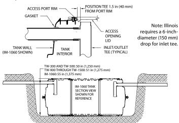
8. Install lids and risers (see Installing Risers section) as necessary.
