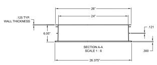
24" x 6" Riser Cutaway
