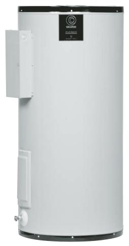
Designed for use as recovery heaters for light-duty hot water supply service. Patriot™ PCE water heaters are available with tank capacities from 6 through 119 gallons. They can be installed for non-simultaneous and single element operation (maximum input up to 6 KW), or for simultaneous dual-element operation (maximum input up to 12 KW).
