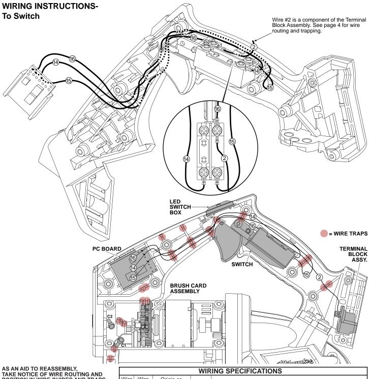
AS AN AID TO REASSEMBLY, TAKE NOTICE OF WIRE ROUTING AND POSITION IN WIRE GUIDES AND TRAPS WHILE DISMANTLING TOOL.
