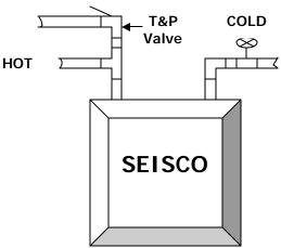
Above diagram shows plumbing connections with a T&P Valve if required by local codes.
