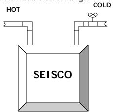
Above diagram shows approved plumbing connections without T&P Valve (T&P NOT REQUIRED BY MANUFACTURERER).
