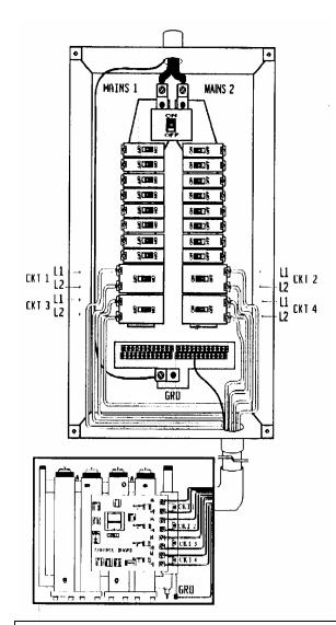
WHERE REQUIRED BY CODE, USE A DISCONNECT SWITCH ADJACENT TO THE WATER HEATER. WHEN MAKING THIS TYPE OF INSTALLATION, BE SURE THE MAIN FEEDER WIRES USED ARE PROPERLY SIZED.
