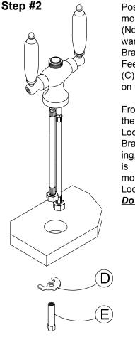
Position the Bar Body over the mounting hole as shown. (Note: The Handles pull forward to turn on.) The Mounting Bracket must be in the back.) Feed the Bar Supply Hoses (C) through the mounting hole on the counter.
