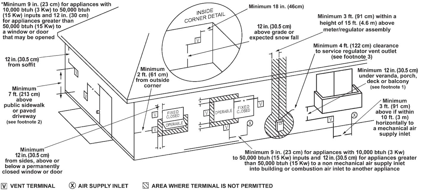
1. Permitted only if veranda, porch, deck or balcony is fully opened on a minimum of two sides beneath the floor.
