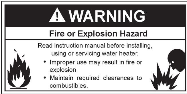
Minimum clearances between the water heater and combustible construction are 0 inch at the sides and rear, 6" (15.2 cm) from the front of the jacket, and 12" (30.5 cm) from the top (standard clearance). If clearances stated on the heater differ from standard clearances, install water heater according to clearances stated on the heater.
