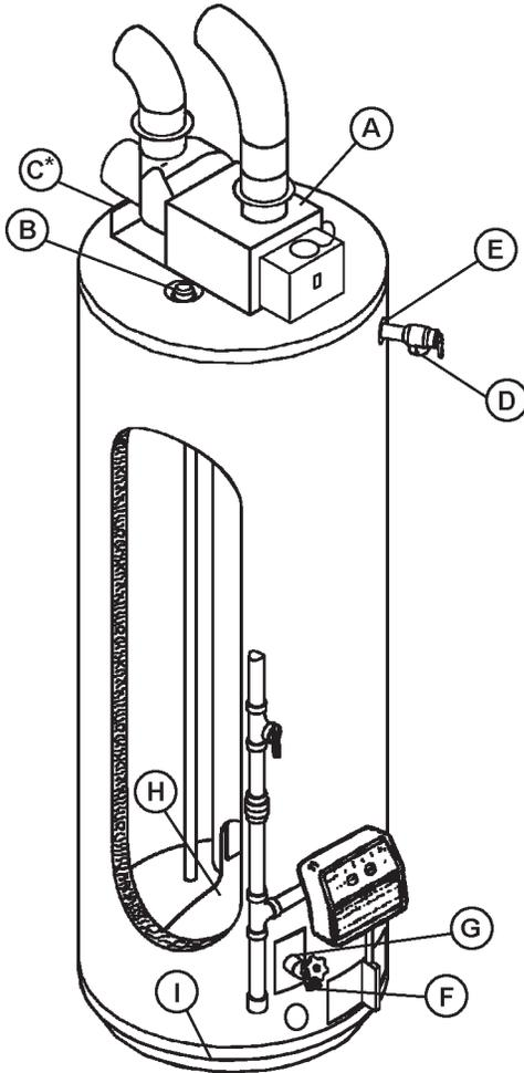
A. Water at the blower assembly is water vapor which has condensed out of the combustion products. This is caused by a problem in the vent. Contact the gas utility.
