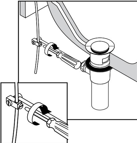
Connect the swivel connector to the end of the ball rod.
