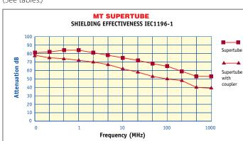
The graphs above show that the shielding effectiveness of MT Supertube is highly effective throughout the entire frequency range and will provide protection from interference for data, telecoms and signal cables.
