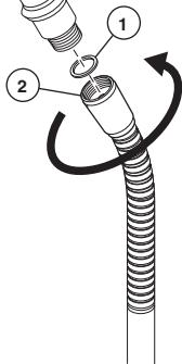
**Connect tapered end of hose to hand shower:** Seat the washer (1) firmly into the hose nut (2). Carefully align the thread of the tapered end of the hose nut (2) directly to the hand shower. **Hand Tighten—do not use a wrench or pliers.** Then place the hand shower into the wall mount holder.
