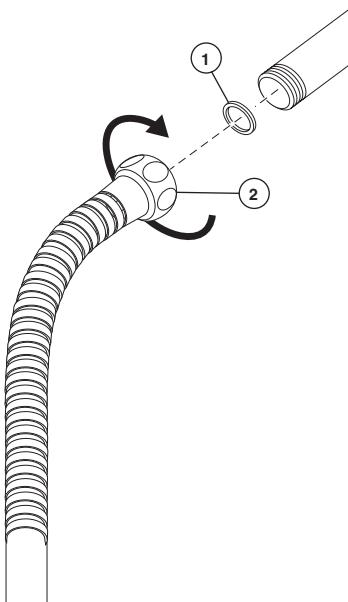
Ensure gasket (1) is inserted into the hose (2). Connect the hose to your designated water supply.
