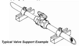
**CAUTION:** All valve connectors and connecting pipe should be inspected for any breaking, chipping, gouging or other visible damage before proceeding. All joining components must be clean and dry. All valves and pipe shall be removed from their packaging or containers and exposed to the environment for a minimum of one hour in order to thermally balance all components. Installation temperatures should be between 40°F and 110°F.
