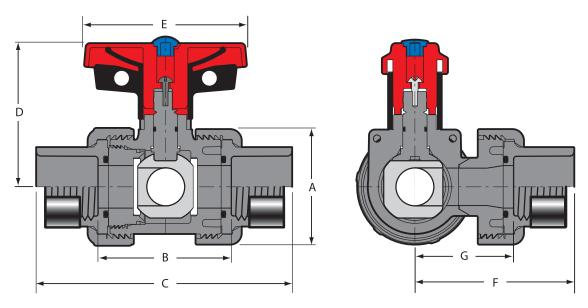
NOTE: Diverter style valve has no shutoff on branch
