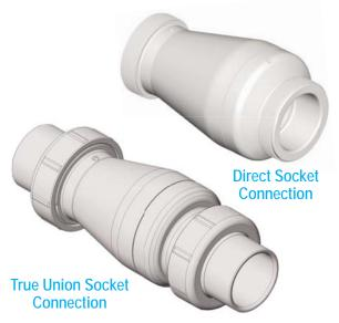
Spears® Quiet Check Valve has been designed to provide quiet operation in sump pump or sewage ejector pump systems typically found in home basements. The back flow of the water column in the discharge pipe can slam conventional check valves closed, producing a disturbing "thump" when the pump shuts off. The Quiet Check Valve uses a spring controlled rate of closing to prevent slamming and eliminates the noise.
