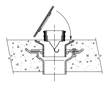
THE 3" TRAP GUARD COMES INSIDE A FLEXIBLE BUSHING THAT WILL FIT MOST 4" STRAINER TAILPIECES OR ANY 4" HUB SIZE OPENINGS, PLASTIC OR CAST IRON.
