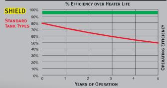
**NOTE:** The chart is based on limescale build-up of 1/16 inch per year which reduces operating efficiency approximately 8-10% per year.
