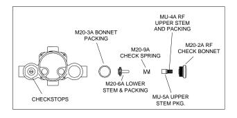
**REMEMBER!** THIS IS A CONTROL DEVICE WHICH MUST BE CLEANED AND MAINTAINED ON A REGULAR BASIS (SEE MAINTENANCE GUIDE AND RECORD)
