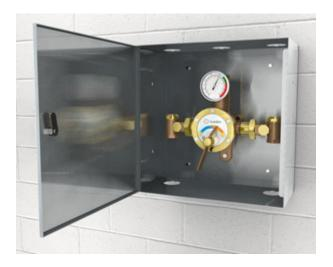
**APPLICATION:** Tempering valve to blend hot and cold water to deliver tepid water. Valve is installed in stainless steel cabinet designed for surface mounting on finished wall. Valve has flow capacity of 3.0 to 44 gallons per minute (GPM). Valve can be used with single installation of emergency showers and safety stations, and with multiple installations of emergency shower, eyewash, eye/face wash, dual purpose eyewash/drench hose, drench hose and safety station units.
