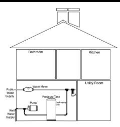
Your new **Aqua-Pure** Water Filter installs on the main cold water line after entering the home. Complete installation instructions included for your convenience.
