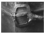
18. Compress gasket at corners with vice-grip while snapping in corner clips.
