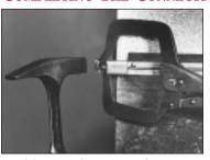
Slide corner clips onto joined corner pieces. Tap with hammer until rear tab clicks into notch on corner pieces and locks in for a permanent connection.
