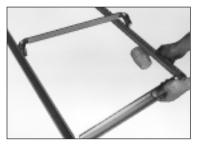
Slide two longer angle pieces onto corner pieces already inserted into shorter pieces, then add the second short piece to complete the frame.
