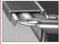
9. The duct must be seated all the way into the Ductmate angle in order to penetrate the integral mastic sealant and avoid leakage. The corner of the duct MUST protrude beyond the Ductmate corner piece.
