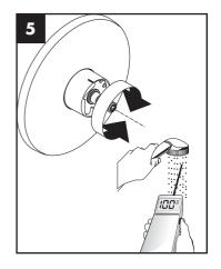
Install the handle so that the safety stop override button is at the 12:00 position, next to the indexing mark on the sleeve.
