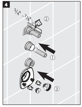
Install the thermostatic cartridge by hand. Tighten to 15 Nm ( $\pm$  2 Nm) using a 24mm wrench.
