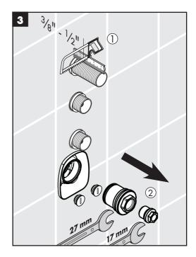
Install the volume control extension spindles (1).
