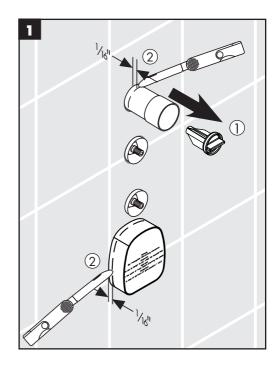
Seal the wall around the plaster shields using waterproof sealant (1).
