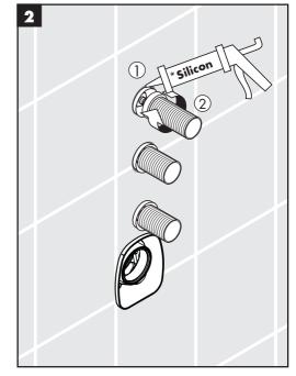
Cut the slip connector so that it extends  $\frac{3}{8}$ " -  $\frac{1}{2}$ " outside the surface of the finished wall (1).
