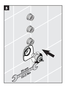
Push the cut extension spindles into the sleeves.
