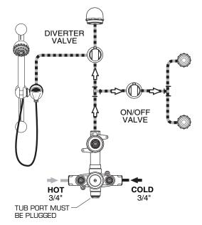
**NOTE:** MINIMUM FLOWING PRESSURE REQUIRED FOR THIS SYSTEM OPERATING WITH ONE SHOWER HEAD AND 2 BODY SPRAYS IS 40 PSI
